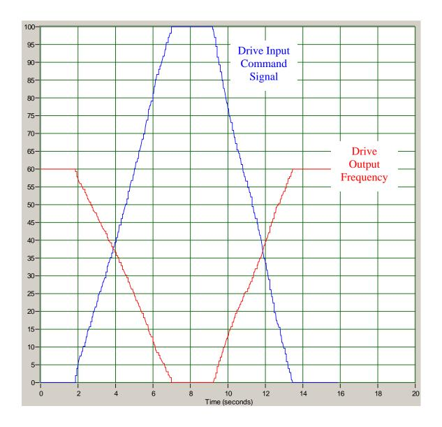
0 input = maximum speed 100% input = 0 speed
