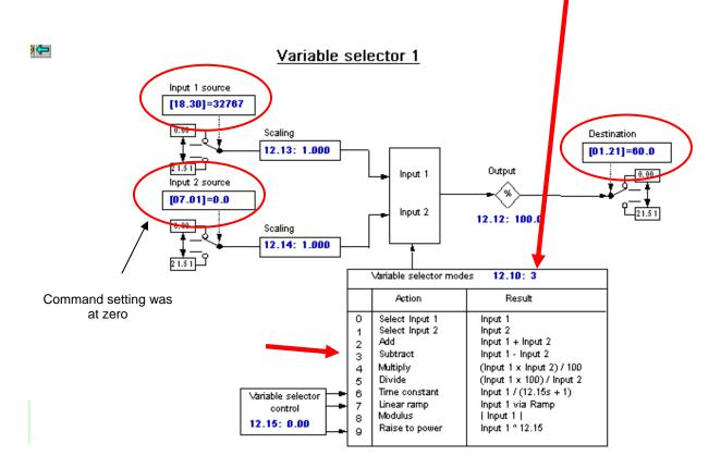
This method will use the facilities of the Variable Selectors of menu 12. This method simply uses the subtract function to accomplish the inversion.
